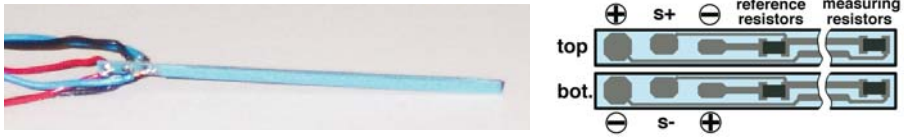
Figure 9. Fired LTCC sensing module (left), and layout of core layers (right). +/- = positive/negative supplies; s + / - = positive/negative bridge outputs (Maeder et al 2007a).
