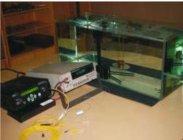
Figure 11. A view of the balance mounted on to the calibration body immersed in water (fish tank).
