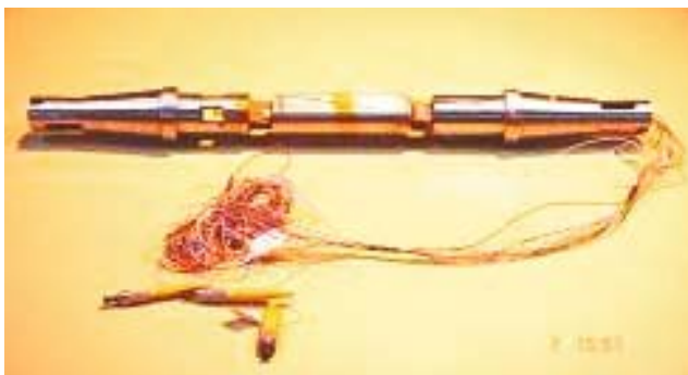
Figure 2. A view of the 6-component strain-gauge balance with both EFPI fibre-optic gauges and conventional strain gauges.
