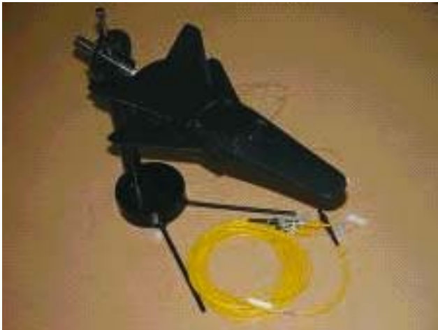
Figure 13. A view of the fibre-optic balance mounted inside the model
