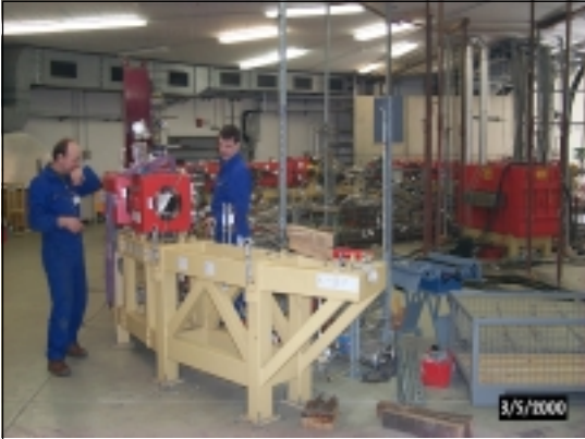
Figure 1. Booster synchrotron under disassembly.
