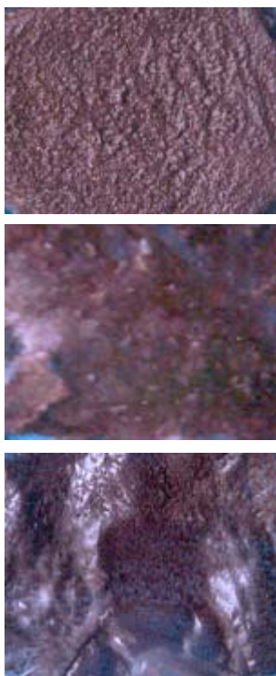
Figure 1. Optical micrograph images of \gamma\text{-Fe}_2\text{O}_3 dispersed (a) natural rubber. (b) polyethylene glycol (c) polycarbonate composite films.
