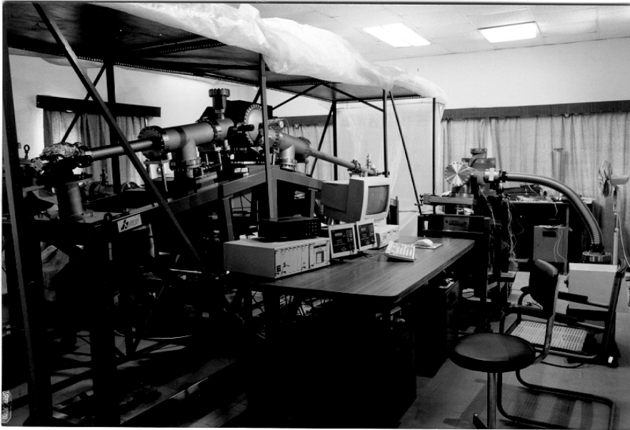
Figure 1. The photograph shows part of the beamline to be put on INDUS-1. The toroidal grating monochromator is seen on the left, the computer controlling the grating angular position is in the front and the post-mirror section is on the right.
