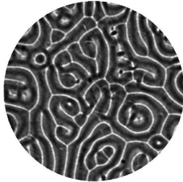
Figure 1. A typical image of the convective state exhibiting spiral defect chaos (at \epsilon = 2.82 ) as visualized using shadowgraphy. The convective fluid is bounded horizontally in a circular domain with radius 3.8 cm and vertically extends to about 0.69 mm.
