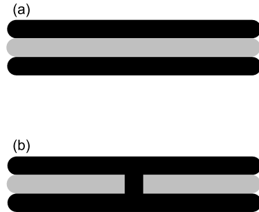
Figure 2. A schematic of roll pinch-off and merger for a set of rolls participating in defect nucleation is shown. During this process, the two dark rolls merge, leading to the number of distinct dark rolls halving from 2 to 1. At the same time, the lighter colored rolls split, doubling their number from 1 to 2. Concurrent with this, the size of the distinct darker roll has approximately doubled while that of the lighter roll has halved. The number of nearest-neighbors in this ideal case of parallel alignment of rolls has also been increased from 1 light roll to 2 light rolls, and vice versa for the dark rolls. The physics of such dynamics therefore motivates studying distributions of roll sizes and nearest-neighbor distributions in base 2.
