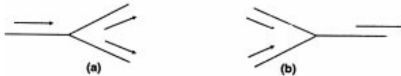
Figure 5. (a) Three port coupler as a splitter. (b) Three port coupler as a combiner.
