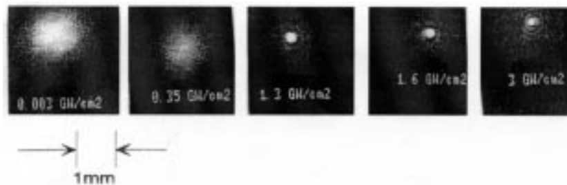
Figure 2. Laser beam transverse section at the output of a CS 2 cell (length 0.5 cm) – excitation provided by a mode-locked Nd:YAG laser (duration 30 ps). Intensity ranging from 3 MW/cm 2 to 3 GW/cm 2 .
