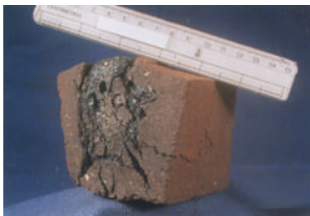
Figure 3. Mixed pond-ash clay bricks obtained on curing at 1200°C showing agglomeration of iron and slag.
