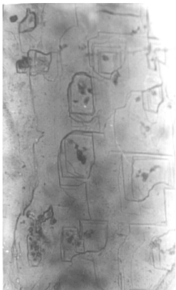
Figure 6. Crystallographically oriented pits on the surface of cholesterol crystal.
