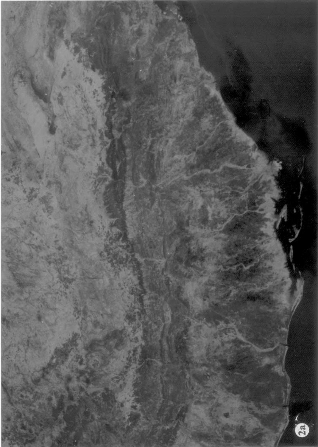
Figure 2(a). Thematic mapper image of the southern part of Kutch region. The greenish gray E-W trending banded formation in the central part of the image is the Deccan Volcanic flows, which are sandwiched between the Mesozoics exposed in the north and Tertiaries in the southern part. A number of flows comprising the Deccan volcanics are in general dipping in the southerly direction. On the eastern side Deccan volcanics can be seen forming a southeasterly plunging anticlinal structure, the eastern limit of which is cut by NW-SE trending strike-slip fault. Remnant of this limb is located in the NW direction and it is concluded that the sinistral strike-slip movement of about 17 km has taken place since the outpouring of Deccan lavas. Similarly on the western side, Deccan volcanics have also moved in dextral strike-slip fashion by approximately 15 to 17 km.
