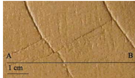
Figure 8. R' shears rotated to a sigmoidal shape and offset as passive markers due to slip along R shears.
