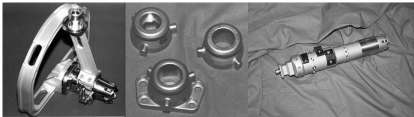
Figure 4. The microconical tool, developed by Oceanering Space Systems in support of the International Space Station (ISS).
