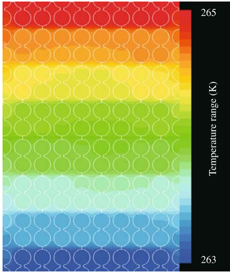
Figure 2. 2-D FE simulation of temperature distribution for unit cell (figure 1a) using Gambit 2.2 and Fluent 6.2. It shows many such cells have been connected vertically to represent a dimension of 26 mm \times 40 mm with lower boundary temperature at 263 K and upper boundary temperature at 265 K.
