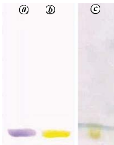
Figure 2. Comparison of relative mobility of annatto dye with bromophenol blue in SDS–PAGE before staining ( a and b ) and after staining ( c ).
