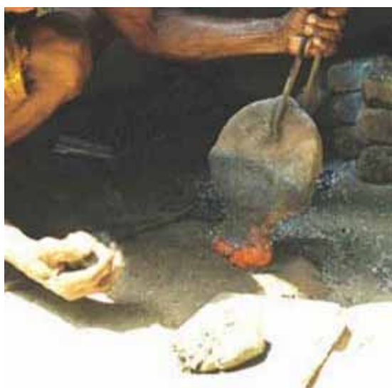
Figure 4. Inverted crucible-cum-mould with the red hot mouth being packed with mud.
