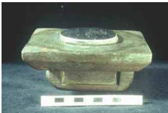
Figure 6. Cast oval (3 mm thick) blank of silvery delta high-tin bronze mounted with heated resin onto a wooden mount, to be polished to get the mirror effect.
