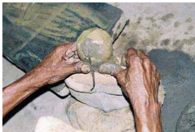
Figure 3. Crucible-cum-mould being sealed with cloth dipped in silt and straw/cotton wick.
