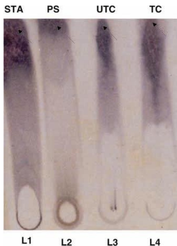
Figure 4. Analysis of tannins in C58-induced transformed callus using thin layer chromatography in T. chebula . STA, Standard tannic acid (lane 1, arrow); PS, Pericarp of seed (lane 2, arrow); UTC, Untransformed callus (lane 3, arrow); TC, Transformed callus showing presence of tannic acid (lane 4, arrow).
