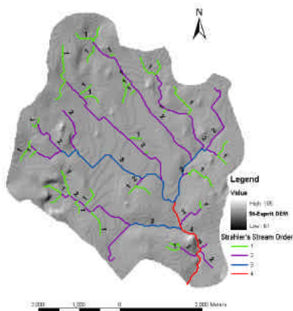
Figure 2. Stream order network of St. Esprit watershed generated using an interface with ArcGIS tool.
