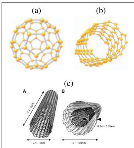
**Figure 2.** Structures of (a) Buckminsterfullerene (b) Carbon nanotube (c) Single walled and Multi walled carbon nanotubes (A) SWNT (B) MWNT
